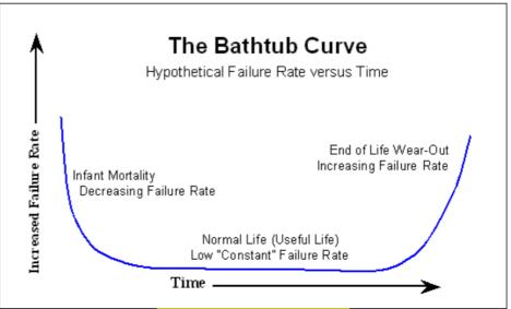
Figure 1: The Typical Bathtub Curve
